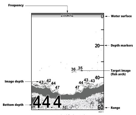
Figure 3-2: Typical Fishfinder Display Screen
